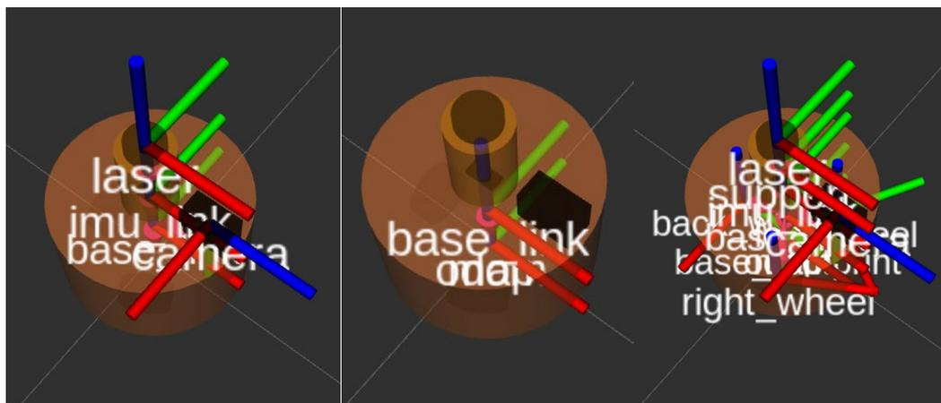
**Figure 4.9 Coordinate transformation setup**
