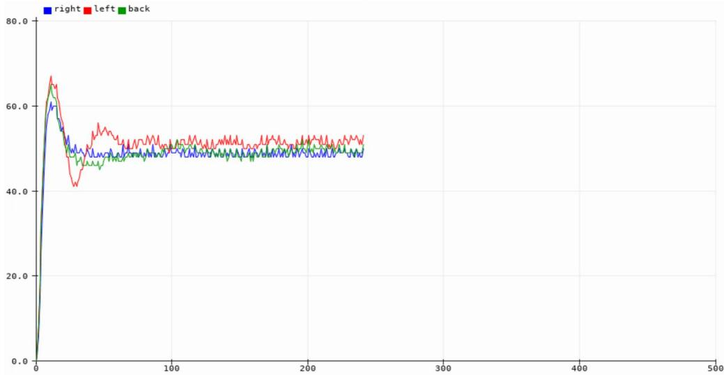
**Figure 4.3 Reduce the value of P by half**
