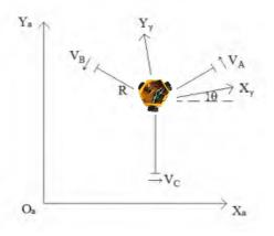
Figure 4.1 3WD robot kinematics
