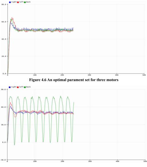
Figure 4.7 Set the parameter I for rear motor
