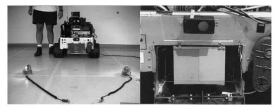
Figure 2.6 Docking devices by Minten et al.
