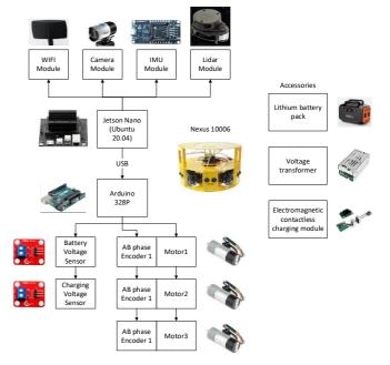
[Figure 1: Hardware structure]
