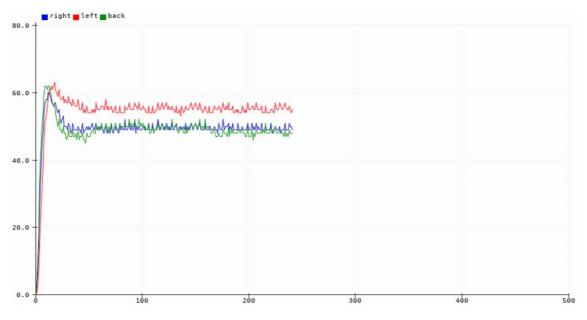
Figure 4.5 First adjustment of D-values for all motors
