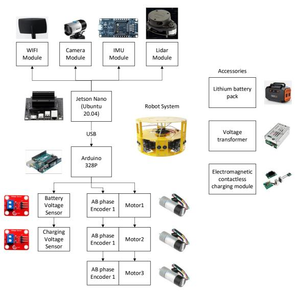
Figure 3.2 Hardware structure
