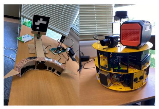
Figure 4.17 Contactless charging module on robot and charging base
