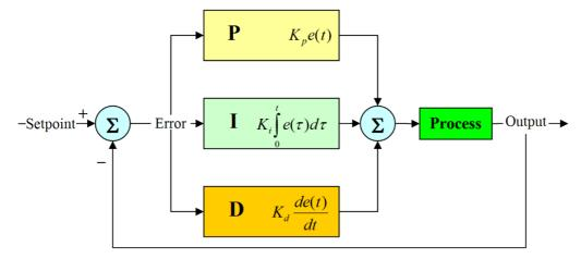
**Figure 2.9 PID controller**
