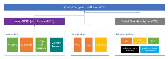
Figure 3.3 Software structure
